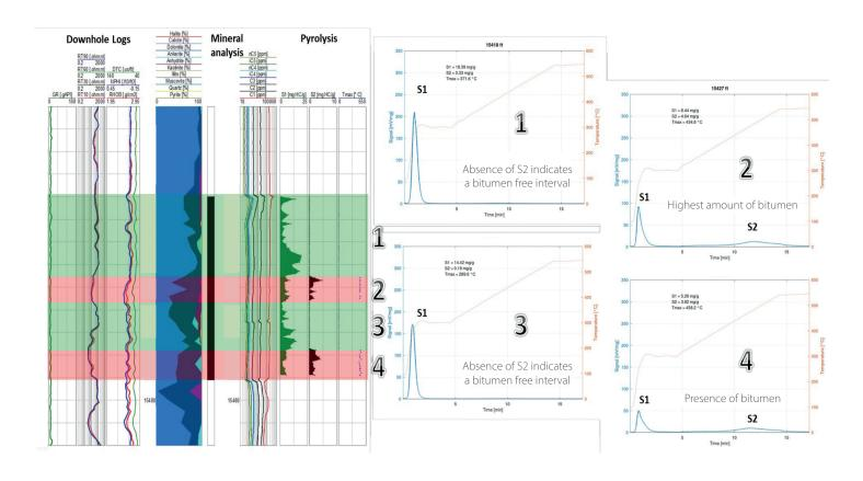
The use of pyrolysis values S2 gives a direct indication of the presence or absence of bitumen within the samples (assuming there is no kerogen present). By identifying bituminous zones, completion design can be adjusted accordingly to isolate problem zones.
