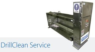
Scales positioned in front of each shale shaker continuously measure in real time the weight of the cuttings coming out of the hole. An engineering software transforms the weights into volume which is graphically displayed on the rig floor. The driller immediately knows what is happening downhole, when cuttings remain in the hole (risk of getting stuck pipes) or when caving occurs .
