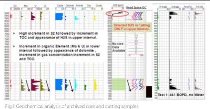
The presence of heavier molecular weight components in the upper interval, associated with an absence of light and intermediate components, suggests the upper interval comprises a very low gravity fluid. The same interval reported high quantities of S2 and TOC.
