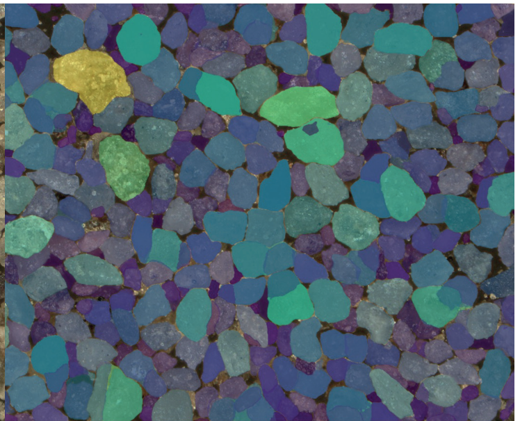
AI segmentation of the same image achieved 99% pixel-wise accuracy in identifying particles
